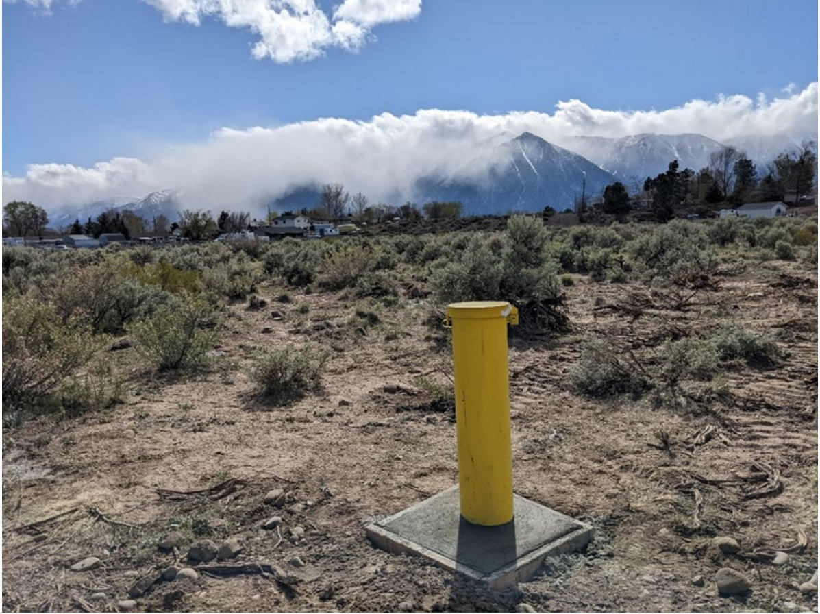
Figure A-5. The completed monitoring well head at MW-3.
